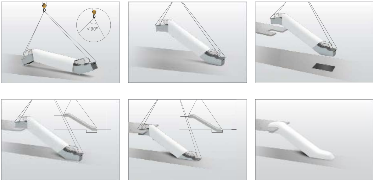
Installation in one complete section by crane
